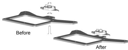
Attach rear pod plate to the center pivot using a 4-40 x 1/2" flat head screw (smr2014). Use a low roll center cone (SMR5008) on top of the lower pod plate, screwing through the 1/4" x 4-40 threaded suspension ball in the center pivot. Secure using a 4-40 mini-locknut (SMR2080) as a jam nut.
